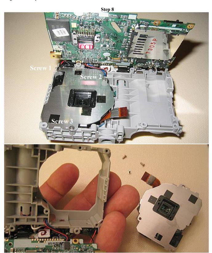
Step 9: Now pry the metal cover plate from the lens assembly. Do this by inserting a small screw driver under one of its three clips, and then twist it. The clip should pop free. Repeat on the other two clips until the plate is removed. Store the plate with its screws in the Step 8 sandwich bag.
