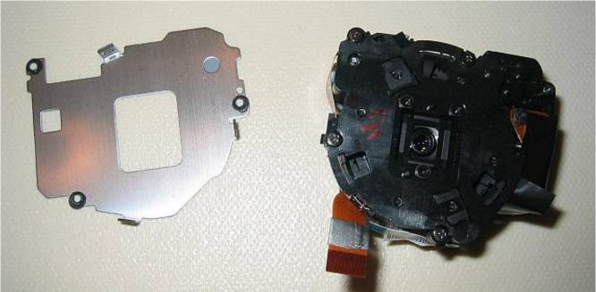
Step 10: Now examine the back of the lens assembly. Remove the four screws that hold its back cover on. Remove the back cover, and store the cover with its screws in a sandwich bag labeled Step 10.
