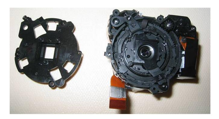
Step 11: Now examine the interior of the lens assembly for any anomalies that may indicate its malfunction. In the below example, two things are apparent. First is that the assembly's guide pins have been dislocated from their intended guide grooves (look at the 4 and 8 O'Clock positions). The second problem is that some of the teeth on the lens assembly's primary gear are missing and damaged (as seen at the 2 O'Clock position)
