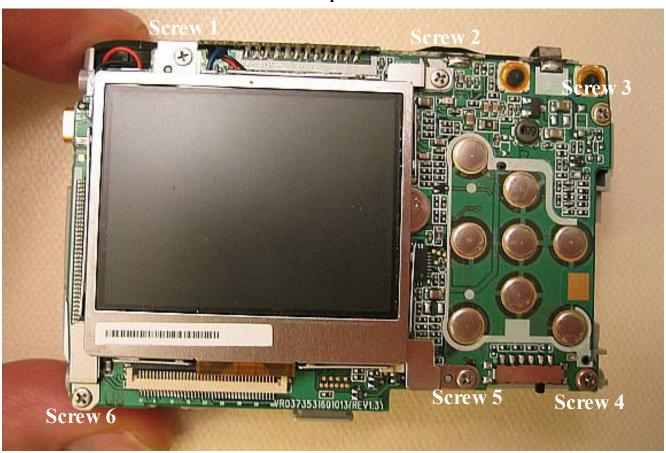
Step 7a: Now gently flip the lcd screen and its metal holding bracket up and over to expose the circuitry beneath it. Do not disconnect the lcd screen's large ribbon cable. But do notice the three small recessed screws, and the smaller ribbon cable and its connector. Remove the three screws and place in a sandwich bag labeled Step 7a.
