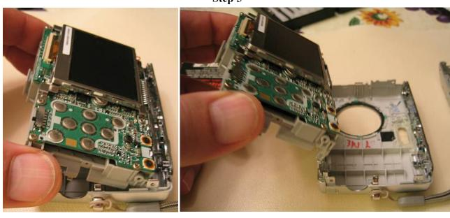
Now take time to examine the electronics assembly. Note the front face with the battery compartment, lens assembly (note that mine is crooked/damaged), autofocus illuminator, and flash assembly. Especially take note of the large green flash capacitor. DO NOT short the terminals of the capacitor to discharge it as you will damage it. Instead recommend slowly draining the capacitor of electricity by applying a voltmeter or some other resistive load until its voltage is discharged (see Step 6b).
