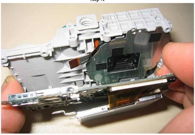
Step 8: Now remove the three screws on the metal cover plate over the lens assembly. Take extra care not to damage any circuit board components, especially the exposed CCD! After the screws are removed, the cover plate and lens assembly should now easily lift out. Store the screws in a sandwich bag labeled Step 8.
