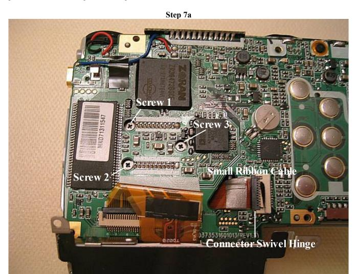
Step 7b: Now notice the black hinge on the small ribbon connector. Swivel this black hinge upward with your finger nail. The small ribbon should now easily pull free. Note that the cable has no connector on its end once it's pulled free.
