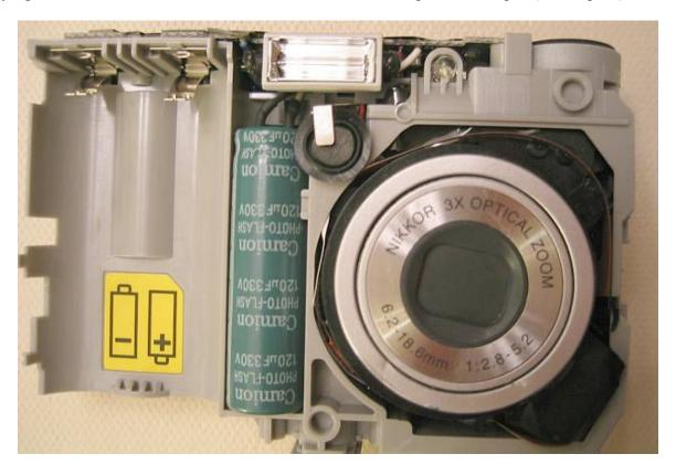
Step 6a: Now examine the top face of the assembly. Note the tape, and the three exposed screws. Remove and temporarily store these three screws.
