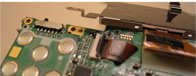
Step 7c: Now very carefully tug and lift the bottom of the circuit board. It should hinge upward as the battery leads bend and serve as the hinge point.
